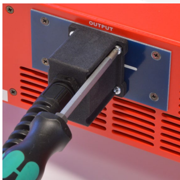
Figure 20: Connect the wire to the output connector
