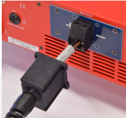
Figure 20: Connect the wire to the output connector
